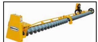
**2000 Series Sweep** — Engineered for heavy farm to light commercial duty. For bin diameters: 30 to 78 feet (9.1 to 23.8 m). Auger diameters: 10 or 12 inches (254 or 305 mm). Capacities range up to 6,500 bushels (165 metric tons) per hour.
