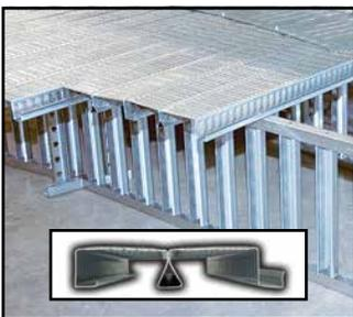
**Brock's TRI-CORR® Bin Aeration Flooring System** combines a unique triangle-shaped center leg with a corrugated flooring surface and PARTHENON® Support Legs to deliver remarkable load-bearing strength, longevity and even air distribution for simple bin clean-out.
