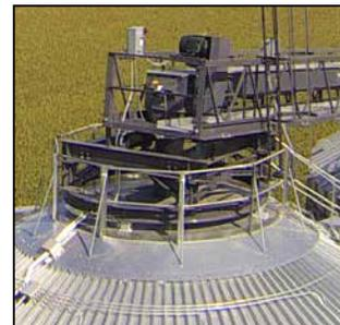
With Higher Bin Roof Peak Loading, it is crucial to safely transfer loads correctly and directly into the roof structure. The Brock EVERLOC® Roof Mount System's support components are attached directly to the roof structure during bin construction to ensure proper load transfers into the structure.
