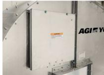
**Head explosion vent** available on all models; Standard on all M42 and M48 models.
